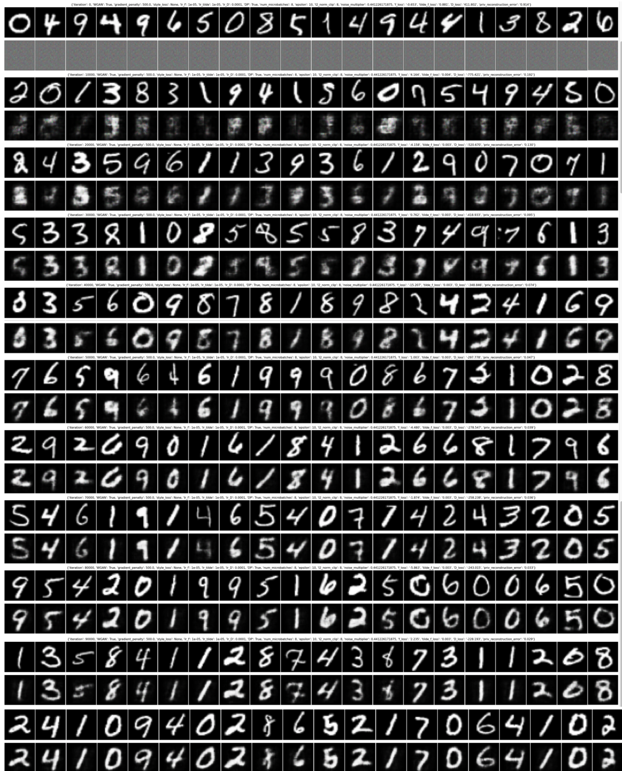
Figure 8: Reconstruction attempts for \epsilon = 10 and 100 000 iterations. Odd rows show the private data fed to the private local f model and the even rows below show the corresponding images reconstructed using attacker's f^{-1} model. The lower the line, the more training iterations there were.
